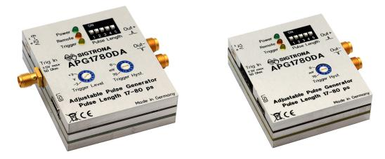
There are two variants: The APG1780DA-SMA has a single-ended  $50\Omega$  terminated SMA input (left) and the APG1780DA-DIFF has a differential input using a SATA connector. The differential input triggers on the zero crossing and hence does not provide means for adjusting a trigger level.
