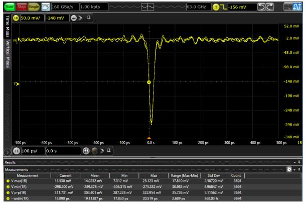
Reducing the pulse width below  $25 \,\mathrm{ps}$  also reduces the amplitude:  $19 \,\mathrm{ps}$  pulse, amplitude  $300 \,\mathrm{mV}$ .
