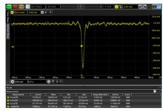
Reducing the pulse width below 25 ps also reduces the amplitude: 19 ps with close to 300 mV.
